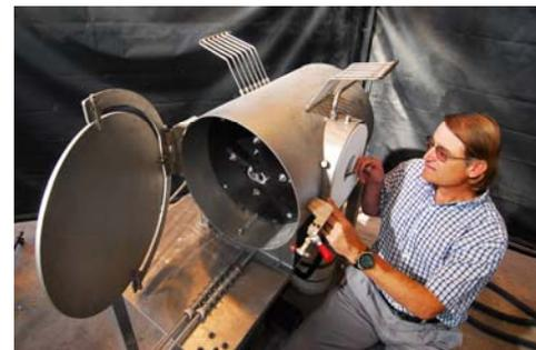
*Above, Sandia researcher Rich Diver assembles a prototype device intended to chemically reenergize carbon dioxide into carbon monoxide, which could ultimately become the building block to synthesize liquid combustible fuels. Photo Credit: Randy Montoya.*
