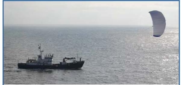
Testing SkySails on a cargo ship.
