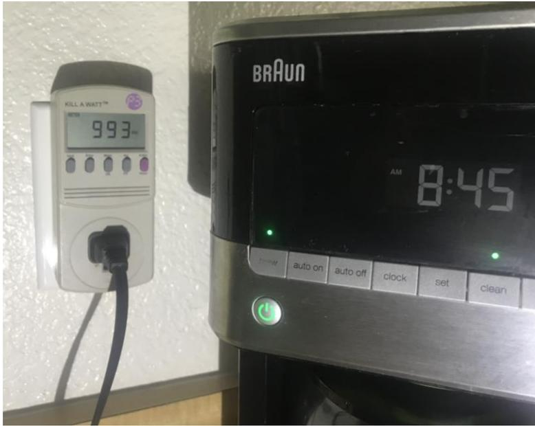
The Kill-a-Watt® meter indicates the power needed for this coffee maker: 993 watts.
