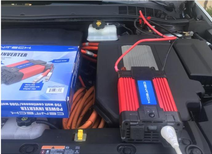
An automotive power inverter connects to the lighter socket in the car or to the car's battery or, for an electric hybrid like this Chevy Volt, to the positive and negative terminals used for jump starting. Refer to your vehicle owner manual for guidance.
