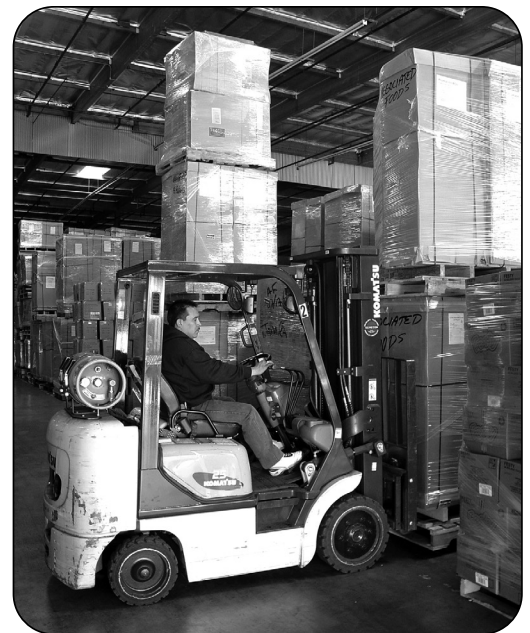
This forklift is fueled by propane.
