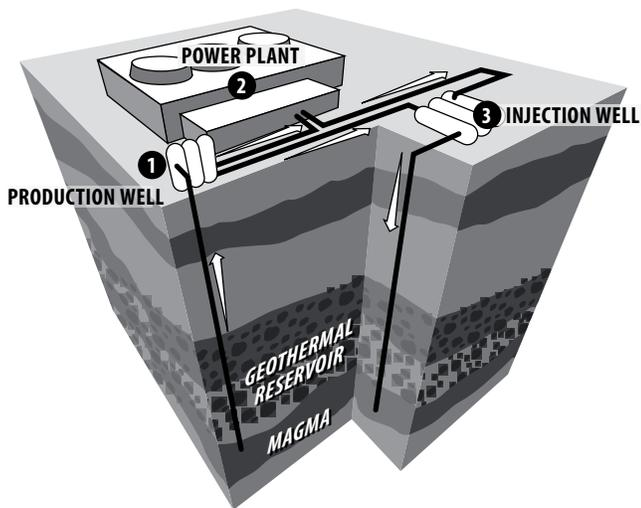
1. **Production Well:** Geothermal fluids, such as hot water and steam, are brought to the surface and piped into the power plant.
