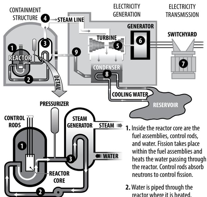
1. Inside the reactor core are the fuel assemblies, control rods, and water. Fission takes place within the fuel assemblies and heats the water passing through the reactor. Control rods absorb neutrons to control fission.
